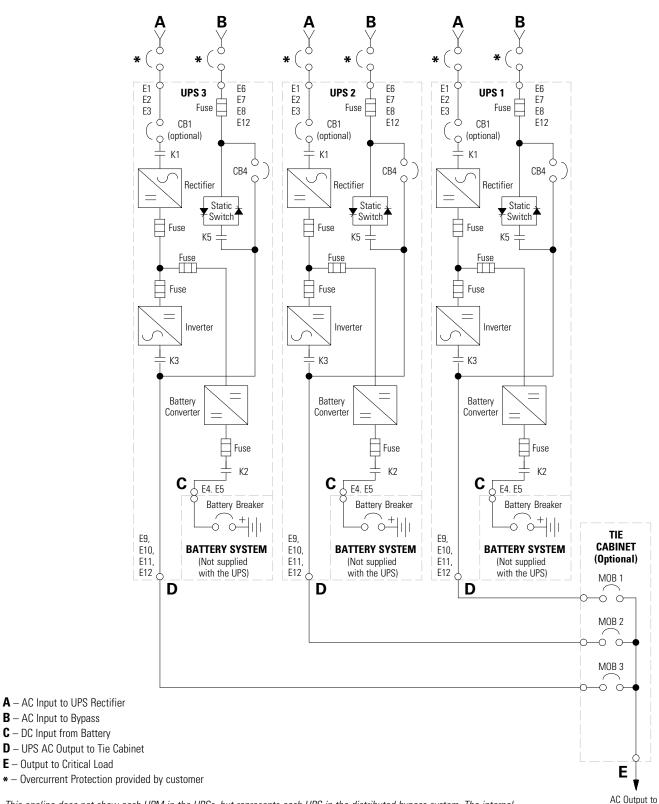
NOTE This oneline does not show each UPM in the UPSs, but represents each UPS in the distributed bypass system. The internal structure of each UPS is shown Figure 6-5 through Figure 6-8 starting on page 6-8.
